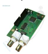
ASI output board is intended for converting the parallel DVB transport stream to DVB-ASI transport stream and can be used for designing a variety of equipment for digital broadcasting
