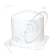
Broadband double reflector antenna with an OMNI directional kind (360 deg. in horizontal plane) of "barrel". Gain: 10 dB, HPBW (vertical): 8 deg. Bandwidth: Ku-band (C-band optional).
