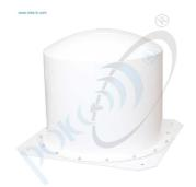
Broadband double reflector antenna with an OMNI directional kind (360 deg in horizontal plane) of "barrel". Gain: 13 dB, HPBW (vertical): 6 deg. Bandwidth: Ku-band (C-band optional).
