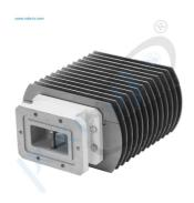
BUC C-band 4W v2 is BUC which operates with up to 25 carriers. Fixed output power P1dB 4 W (400 mW ALC power). Inbuilt reference 10MHz and ALC with 25 dB range. At the rear side BUC has LEDs status indication. The device has integrated matched CWT.
