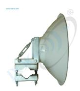
DRA-Ku04 v2 is a double reflector RRS antenna (Cassegrain antenna) Ku-band. Size: 0.4m, Gain: 30dBi, Cross-polarization isolation: 25dB.
