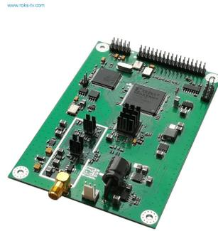
DVB-C/T/S modulator board is designed for converting the parallel DVB transport stream to satellite IF signal, modulated according to DVB-S standard or directly to the RF signal of the DVB-C or DVB-T standards.
