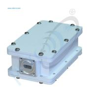
LNB-KaPxx v1 is a PLL LNB with single local oscillator and single 750hm F-type output. LO instability  $\pm$  250 kHz, Gain 50dB, Noise figure 3.5 dB, Output power P1dB +5 dBm.
