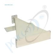
SSA-CV60 v1 - Short Sector Antenna C-band V-pol 60 degree. Features: light weight, compact size, high gain. Beam (H): 60 deg; Beam (V): 20 deg; Frequency range: 3.94 - 5.99 GHz; Gain: 10 dB.
