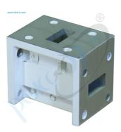
WR75 1/2 (2-way) E-plane power divider v.1 is waveguide tee intended for equal dividing of transmitted or received Ku-band signal between 2 antennas or other blocks.
