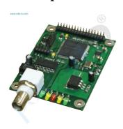
ASI input board is intended for converting the DVB-ASI transport stream to DVB parallel transport stream and can be used for designing a variety of converters and other digital television equipment.
