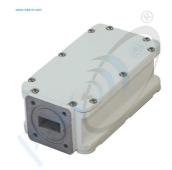
Block Up-Converter Ku-Band 0.2W v2 is BUC which operates with up to 25 carriers. Fixed output power P1dB 0.2W (30 mW ALC power). Inbuilt reference 10MHz and ALC with 25dB range. At the rear side BUC has LEDs status indication.
