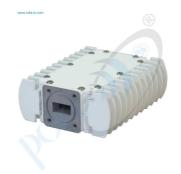
Block Up-Converter Ku-band 1W v2 is BUC which operates with up to 25 carriers. Fixed output power P1dB 1W (100 mW ALC power). Inbuilt reference 10MHz and ALC with 25dB range. At the rear side BUC has LEDs status indication.
