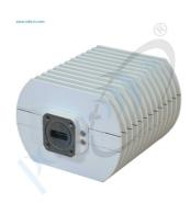
Block Up-Converter Ku-band 10W v2 is BUC which operates with up to 25 carriers. Fixed output power P1dB 10W (1000 mW ALC power). Inbuilt reference 10MHz and ALC with 25dB range. At the rear side BUC has LEDs status indication.
