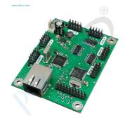
Control board 6ch is used for management and monitoring of various digital broadcasting equipment through TCP /  $\rm IP$
