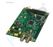
DVB-S/S2 FTA receiver board is designed for converting the satellite IF signal modulated according to DVB-S2 and DVB-S standards to parallel DVB transport stream.
