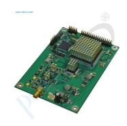
DVB-S/S2/T modulator board is designed for converting parallel DVB transport stream to satellite IF signal modulated according to DVB-S2, DVB-S or DVB-T standards.
