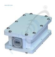
LNB-KPxx v1 is a PLL LNB with single local oscillator and single 750hm F-type output. LO instability ± 25 kHz, Gain 50dB, Noise figure 1.6 dB, Output power P1dB +5 dBm.
