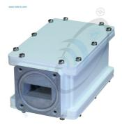
LNB-XPxx is a PLL LNB with single local oscillator and single output. LO instability  $\pm$  25 kHz, Gain 60dB, Noise figure 0.8 dB, Output power P1dB +5 dBm.
