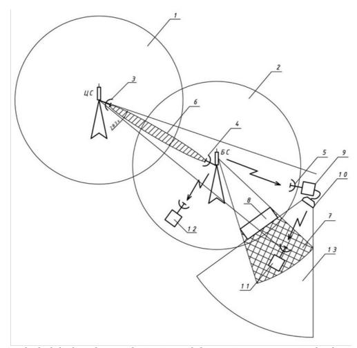
Fig.1 The method of shadowed areas elimination and the service zone expansion by the co-channels repeaters using
