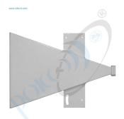
SSA-KuH180 v2 - Short Sector Antenna Ku-band H-pol 180 deg. Features: light weight, compact size, high gain. Beam (H): 180 deg; Beam (V): 16 deg; Frequency range: 10.7 - 13.5 GHz; Gain: 9 dB.
