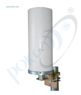
Ku-band OMNI slotted waveguide antenna is designed for MVDS/MMDS broadcasting systems at Ku-band range. It has 360 deg pattern, 1 GHz bandwidth and high Gain 12 dBi.
