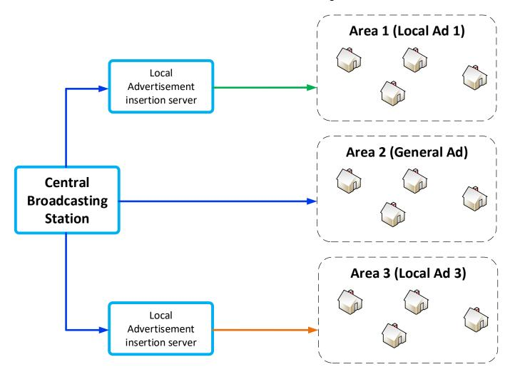
ROKS offers a turnkey software-based solution that allows automatic local content insertion, ticker and animated captions overlaying using DTMF tones or SCTE-104/35 marks in DVB SPTS/MPTS/T2MI or SDI stream. DTMF or SCTE-104/35 should be provided by playout on the central station (not included to our system).
